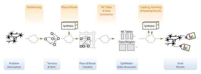
Most SpiNNaker applications provide a domain-specific API for describing whatever is to be simulated. This description is then *partitioned* into a graph of SpiNNaker-core-sized (*vertices*) which communicate with each other (via *nets*). This first step is usually very application specific and so Rig does not provide any functions to help.
