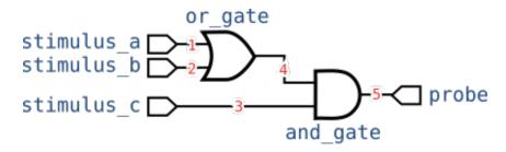
To do this we'll need 6 SpiNNaker cores (one for each gate, probe and stimulus). We'll arbitrarily use the following assignment of cores:
