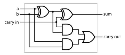
For example if we set 'a' and 'carry in' to 1 and set 'b' to 0, the full-adder circuit will produce a 0 on its 'sum' output and a 1 on its 'carry out' output. Our inputs here are asking the full adder to compute "1 + 0 + 1" to which it dutifully answers "10" ("2" in binary).
