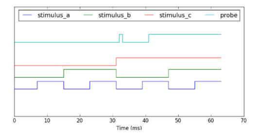
**Note:** The recording shows a 'glitch' at time=32 which is caused by propagation delays in our circuit rather than a bug in our simulator. In fact, our simulator has accurately modelled an unintended feature of our circuit!
